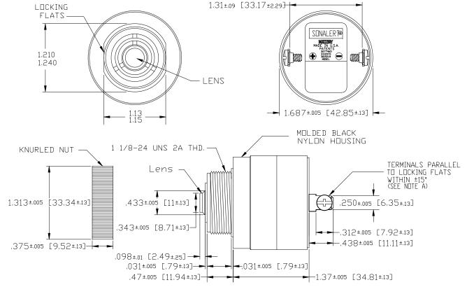
NOTE A: TERMINALS-.032 BRASS TIN PLATED, TAPPED FOR #6-32 TWO #6-32 NICKEL SCREW. PLATED BRASS SCREWS INCLUDED, WILL ACCEPT 1/4" QUICK CONNECT.
